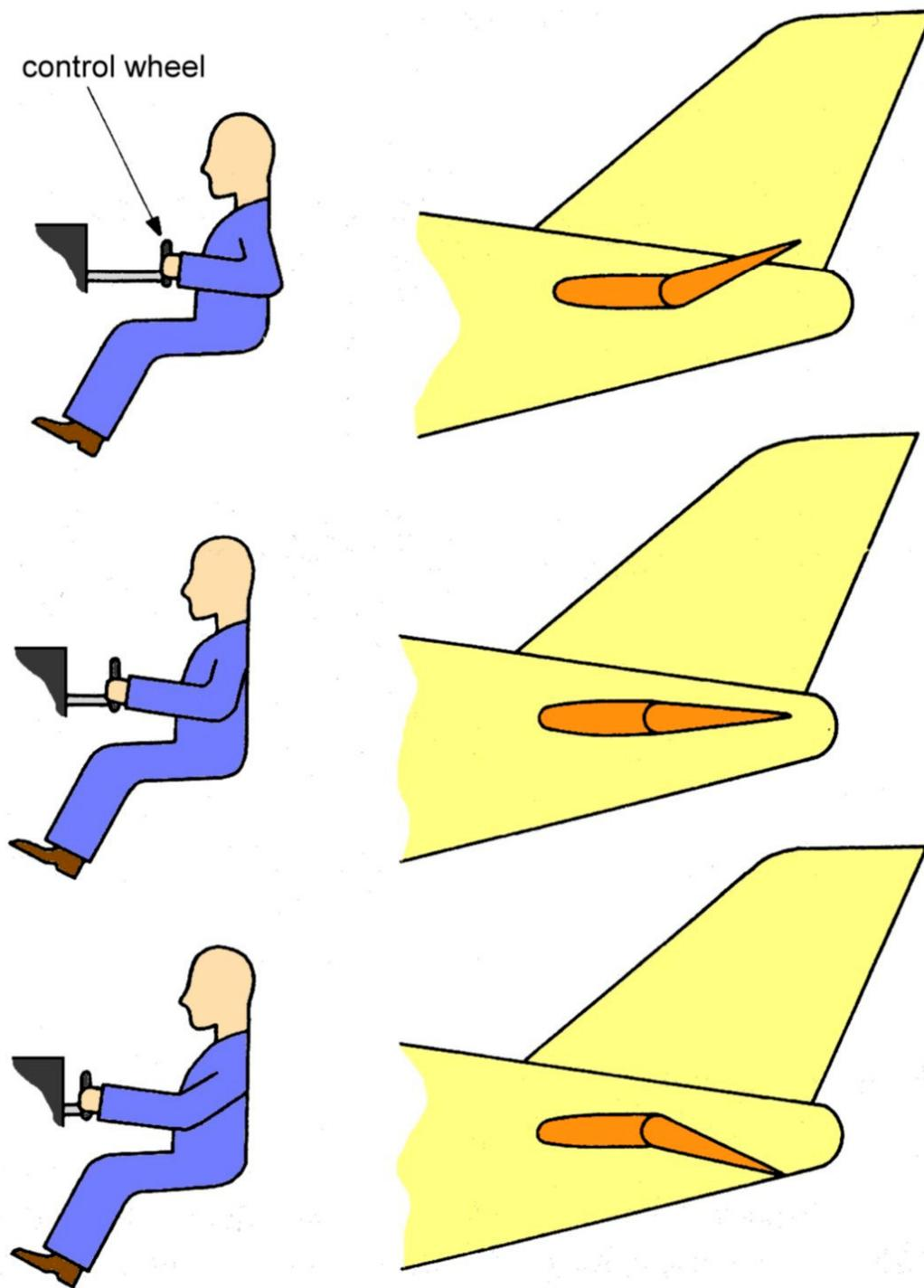
FIG 4. Elevator control
