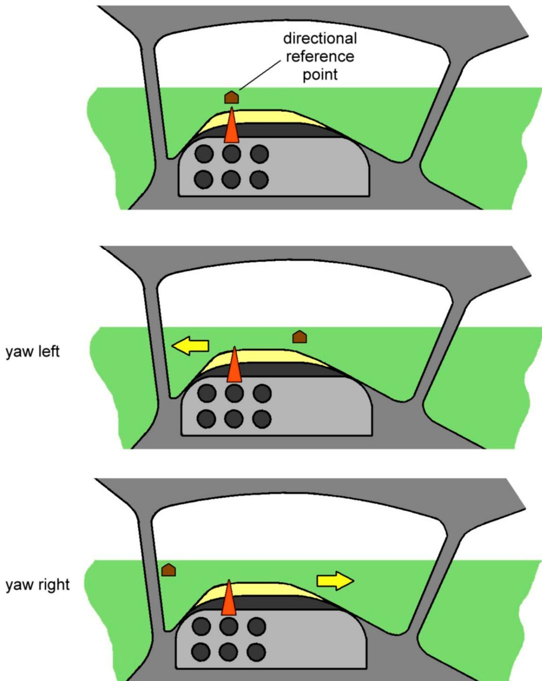
FIG 10. Effect of rudder
