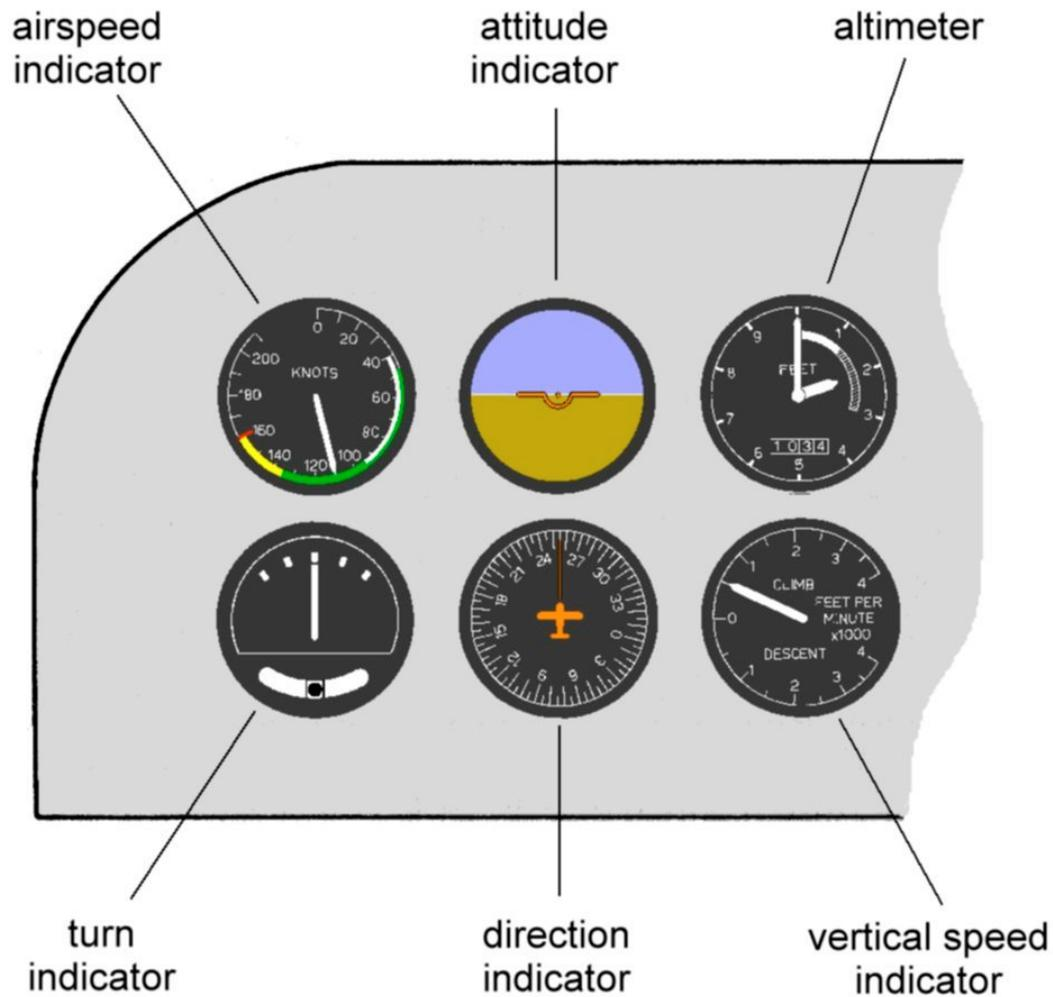
FIG 3. Flight instruments
