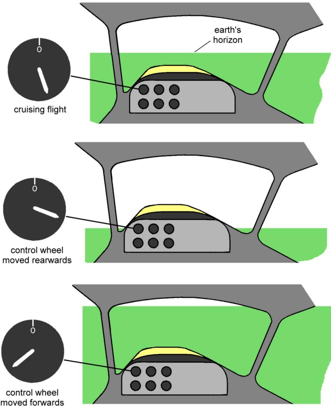
FIG 5. Effect of elevators
