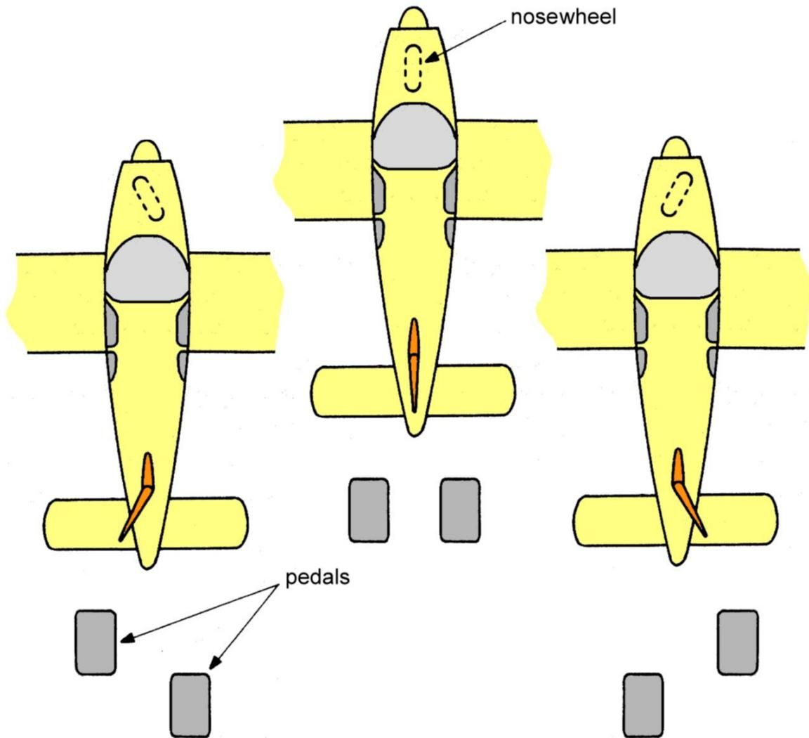
FIG 9. Rudder control and nosewheel steering (view from above)
